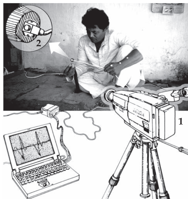
Figure 4.7. Experimental setting, data recordings: 1) a video camera is situated in the axis of the movement; 2) an uniaxial accelerometer is attached to the head of the hammer, and data are recorded via a portable computer.
